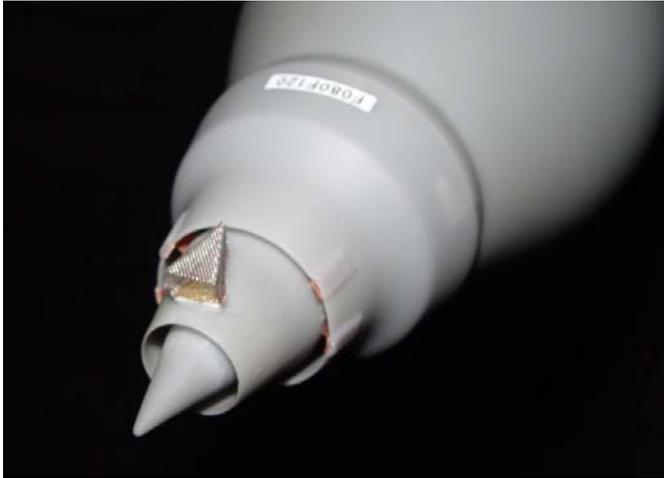
Fig. 13 Photograph of porous wedge deflector.
