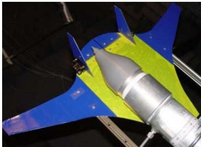
Fig. 2 Installation of nozzle and HWB shield.
