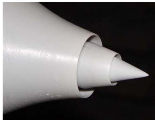
Fig. 3 Coordinates and picture of BPR10 nozzle
