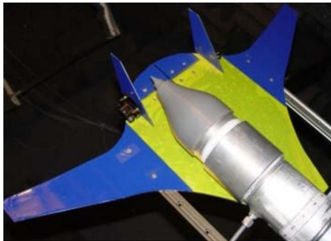
Fig. 2 Installation of nozzle and HWB shield.
