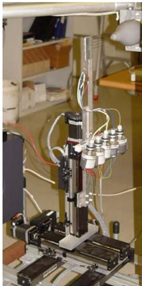
Figure 9. The Pitot traverse system in the Supersonic Mean Flow Facility.
