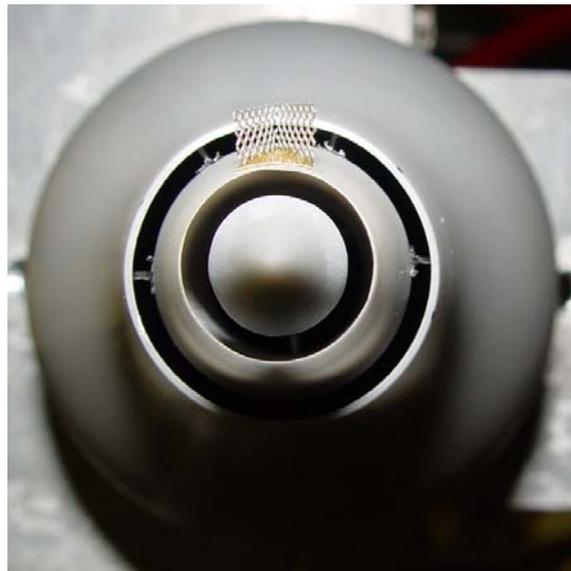
Figure 19. Cambered 4-vane and mesh wedge configuration.
