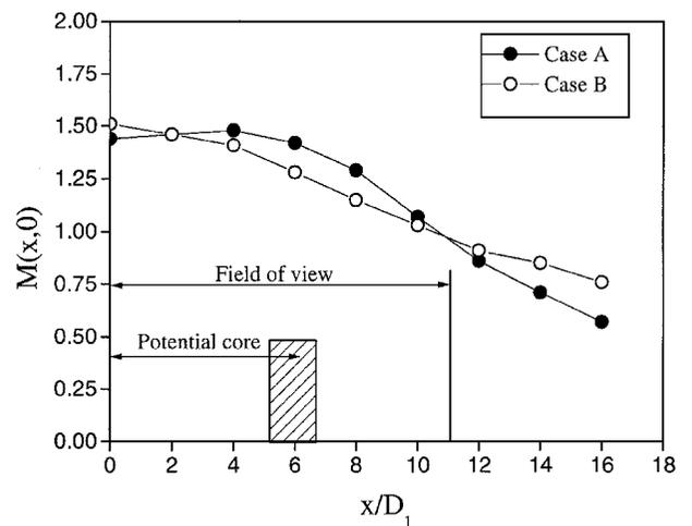
Fig. 5 Centerline Mach number distributions for cases A and B.
