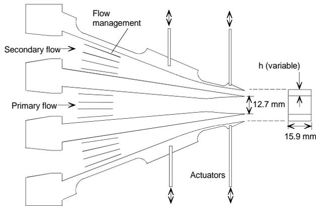
Fig.19 Rectangular dual-stream jet apparatus with secondary flow of variable exit height and adjustable nozzle shape. Upstream actuators controlled the exit height; downstream actuators controlled the nozzle shape.
