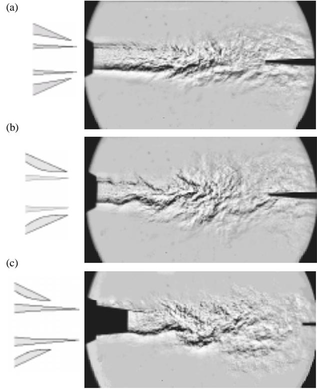
Fig.15 Schlieren images of Mach-0.9, 465-m/s helium-air jets: (a) coflow issuing from a convergent annular duct; (b) coflow issuing from a convergent-divergent annular duct with  $A_e/A_{min}=1.25$ . (c) coflow issuing from a recessed convergent-divergent annular duct with  $A_e/A_{min}=1.35$ . The mass flow rates were approximately equal in all cases. Centerline Mach number at  $x/D_1=8$  dropped from 0.73 in (a) to 0.58 in (b) to 0.52 in (c).
