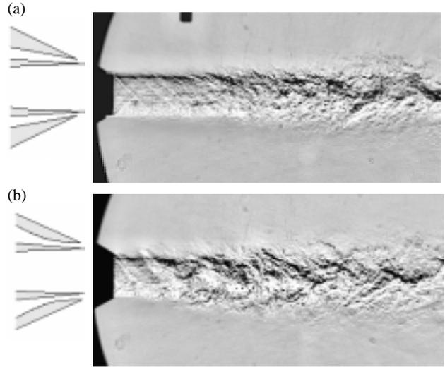
Fig.18 Schlieren images of Mach-1.5, 450-m/s air jets with very thin coflow annulus: (a) coflow duct is convergent; (b) coflow duct is convergent-divergent with  $A_e/A_{min}=1.3$ . Both flows have equal mass flow rate. Centerline Mach number at  $x/D_1=10$  dropped from 1.34 in (a) to 1.04 in (b)
