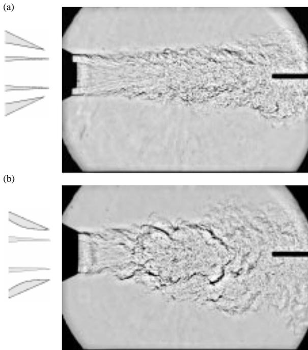
Fig.12 Schlieren images of large annular jets composed of a helium-air mixture. Ideally-expanded Mach number was 0.9 and velocity was 420 m/s for both jets. (a) Annular nozzle is convergent; (b) annular nozzle is convergent-divergent, with  $A_e/A_{min} = 1.11$ . The two jets had the same mass flow rate. Centerline Mach number at  $x/D_2 = 4.7$  dropped from 0.77 in (a) to 0.63 in (b).
