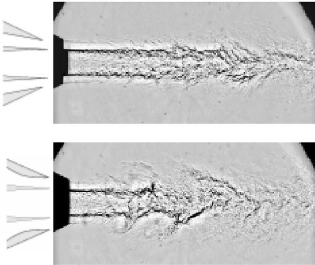
Fig.17 Schlieren images of Mach-0.9, 450-m/s air jets with large coflow annulus: (a) coflow duct is convergent; (b) coflow duct is convergent-divergent with  $A_e/A_{min}=1.1$ . Both flows have equal mass flow rate. Centerline Mach number at  $x/D_1=10$  dropped from 0.76 in (a) to 0.63 in (b).
