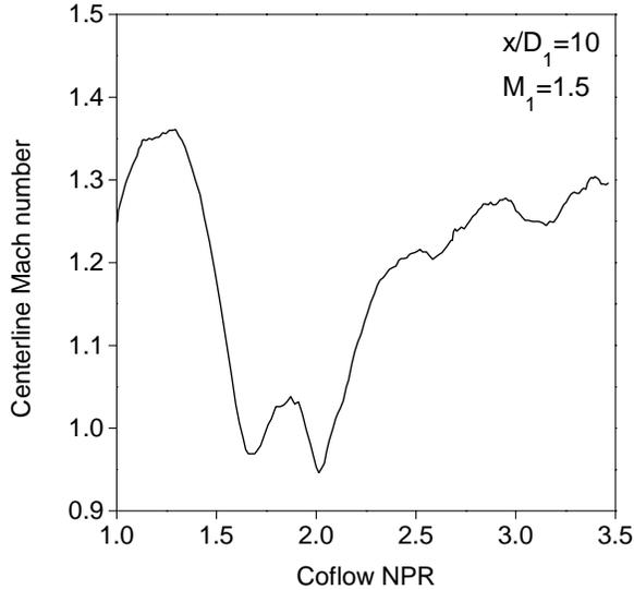
Fig.8 Centerline Mach number at  $x/D_1 = 10$  versus coflow NPR for the arrangement of Fig. 5(c). Inner flow is a Mach 1.5 air jet.
