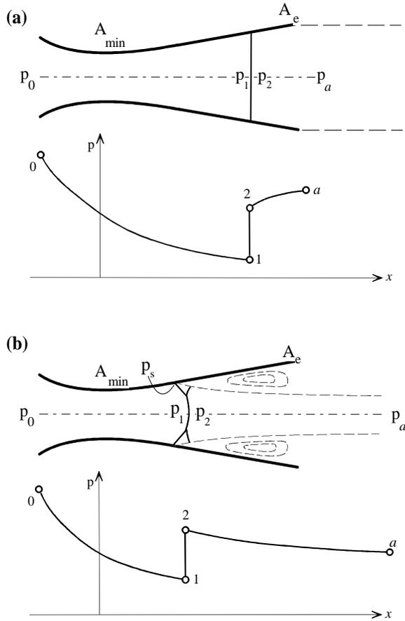
Fig.23 Sketch of shock structure, fluid phenomena, and centerline pressure distributions for overexpanded nozzle. (a) Inviscid case; (b) viscous (separated) case, depicting the under-expansion postulated by Romine [36]. The two cases are compared qualitatively at the same nozzle pressure ratio  $p_0/p_a$ .
