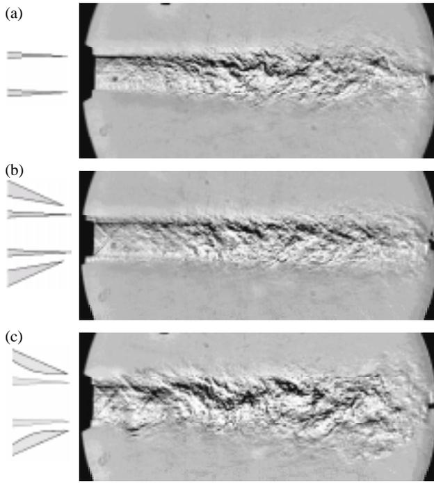
Fig.5 Schlieren images of Mach-1.5, 450-m/s air jets: (a) no coflow; (b) coflow issuing from a convergent annular duct; (c) coflow issuing from a convergent-divergent annular duct with  $A_c/A_{min}=1.25$ . The combined flows have 40% larger mass flow rate and 30% higher thrust than the single jet.
