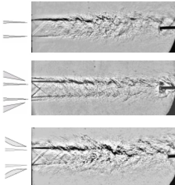
Fig.20 Schlieren images of rectangular Mach-1.5, 450-m/s air jets: (a) no coflow; (b) coflow issuing from a convergent annular duct; (c) coflow issuing from a convergent-divergent annular duct with  $A_e/A_{min}=1.3$ . The combined flows have 33 % larger mass flow rate and 25 % higher thrust than the single jet.
