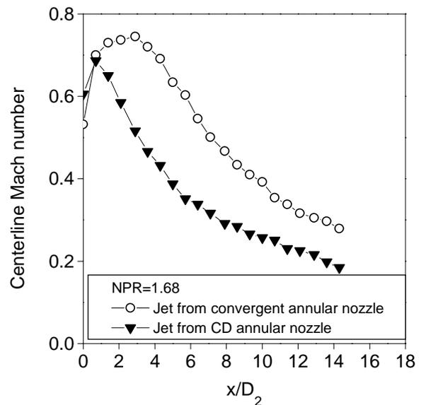
Fig.10 Centerline Mach number distributions for annular air jets issuing from a convergent nozzle and from a convergent-divergent nozzle. NPR= 1.68 and the mass flow rate was equal for both jets.
