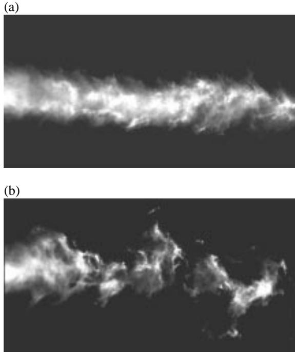
Fig.6 PLIF images of the flows of (a) Fig. 5(a); and (b) Fig. 5(c). Field of view is six jet diameters wide and starts six jet diameters downstream of the nozzle exit.
