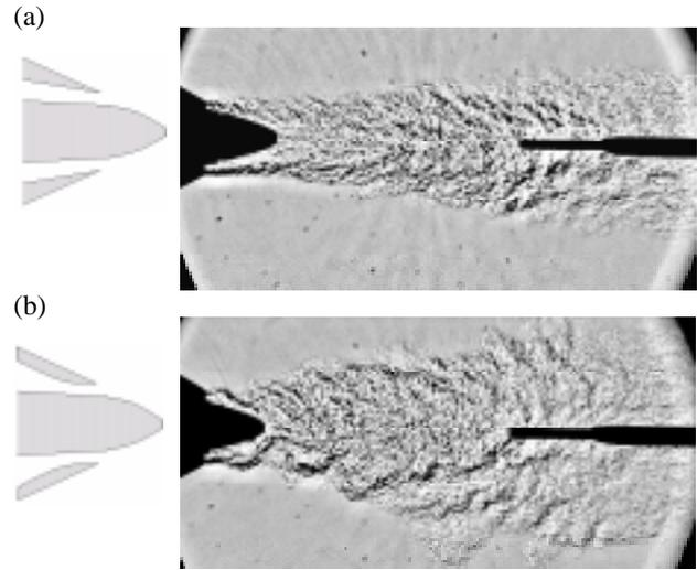
Fig.9 Schlieren images of annular jets composed of a helium-air mixture. Ideally-expanded Mach number is 0.9 and velocity is 410 m/s for both jets. (a) Annular nozzle is convergent; (b) annular nozzle is convergent-divergent with  $A_e/A_{min} = 1.25$ . The two jets had the same mass flow rate. Centerline Mach number at  $x/D_2 = 4.2$  dropped from 0.77 in (a) to 0.48 in (b).
