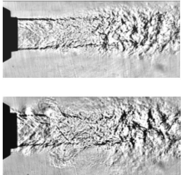
Fig.1 Effect of an annular, unstable coflow on a Mach 1.5 jet.
