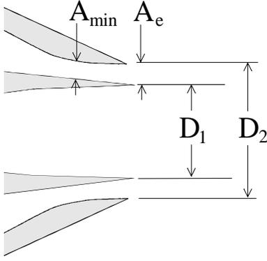
Fig. 3 Generic shape of mixing-enhancement nozzle. Outer (coflow) duct is convergent-divergent. The coflow pressure ratio is such as to cause sonic velocity at the minimum area of the duct and an adverse pressure gradient near the exit of the duct. The properties of the inner steam are irrelevant to the mechanism of the instability.
