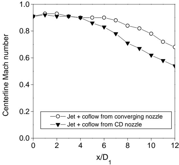
Fig.16 Centerline Mach number distributions for Mach 0.9 air jets with coflow at NPR=1.61 issuing from convergent and convergent-divergent annular nozzles. The setup is the same as in Figs. 15 (a) and (b), except that the jet is composed of air.
