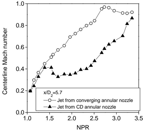
Fig.11 Centerline Mach number at  $x/D_2 = 5.7$  versus NPR for annular air jets issuing from a convergent nozzle and from a convergent-divergent nozzle. At each NPR, the two jets had the same mass flow rate.
