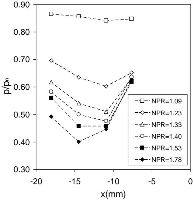
Fig.14 Static pressure distribution on the outer wall of the inner nozzle of Fig. 2(e). Axial distance is measured from lip of inner nozzle. Annular nozzle supplying coflow terminated at  $x = -5$  mm. The data for  $NPR=1.78$  correspond closely to the flow shown in Fig. 13(b).
