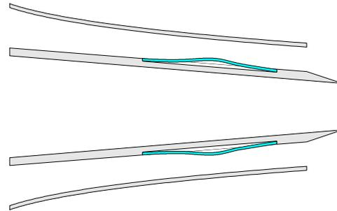
Fig.26 Variable geometry throat for on-demand application of MESPI. Actuation could be pneumatic or mechanical.
