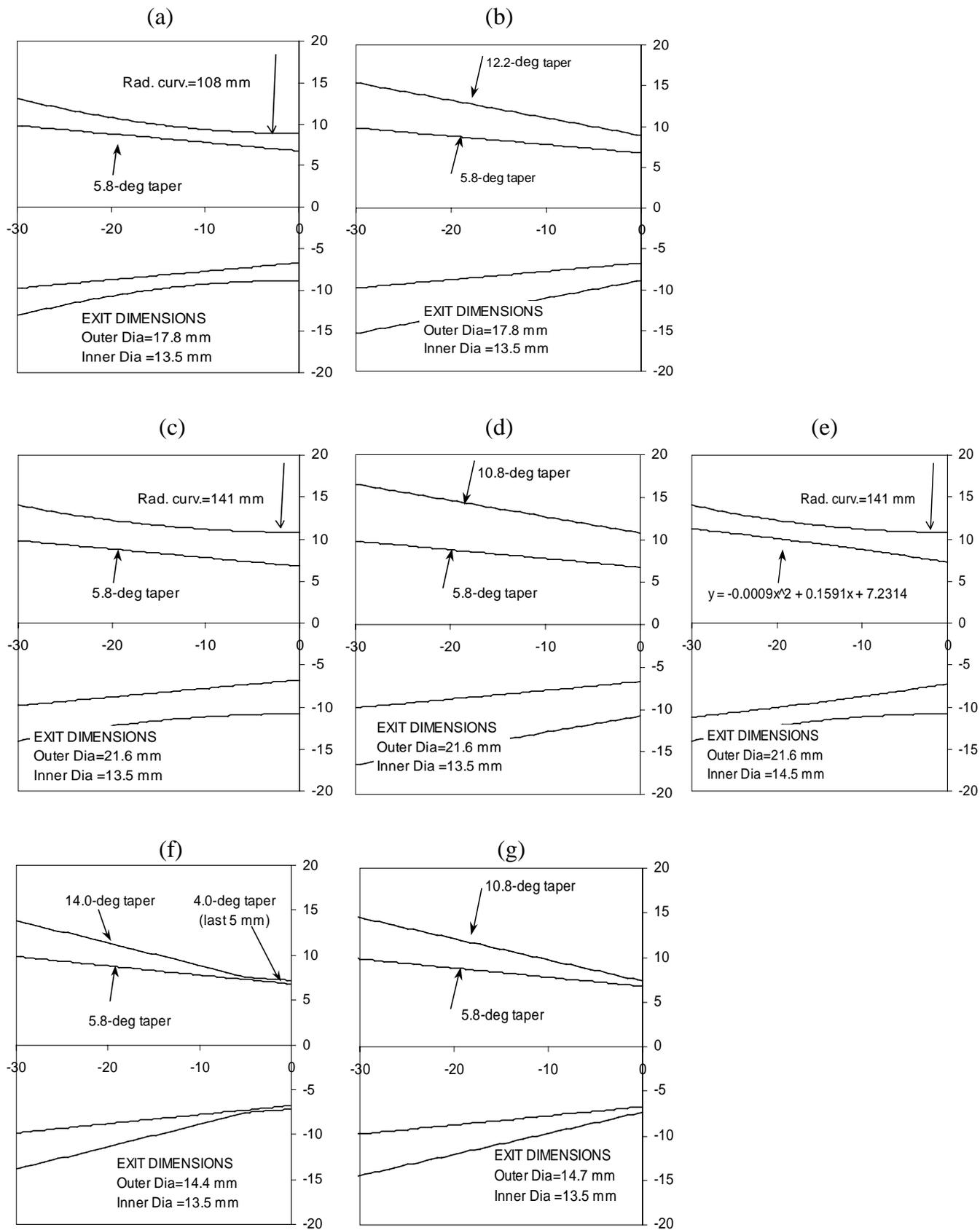
Fig.2 Radial coordinates of axisymmetric coaxial nozzles used in the UCI tests. Dimensions are in millimeters. All arrangements except 2(e) featured the same inner nozzle whose inner duct, not shown, was designed for Mach 1.5 flow. First column: convergent-divergent coflow nozzles; second column: counterpart convergent nozzles; third column: special arrangement using the outer nozzle of 2(c) but a different inner nozzle with constant-area inner duct.
