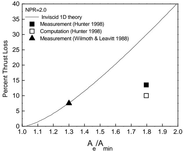
Fig.25 Percent thrust loss versus nozzle area ratio for NPR=2.0. Symbols denote experimental and computational data. Line represents the one-dimensional, inviscid prediction, which is believed to be physically and quantitatively inaccurate.
