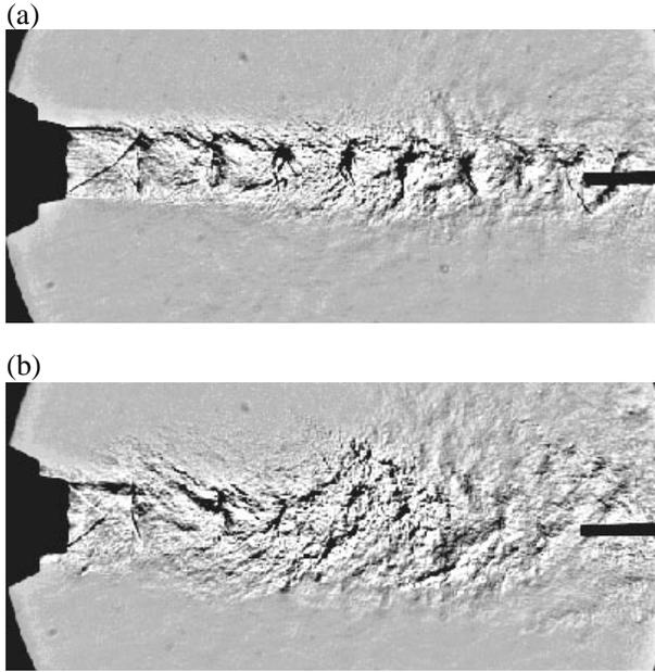
Fig.13 Schlieren images of an underexpanded sonic jet supplied at  $NPR=3.2$  (a) alone and (b) surrounded by coflow from convergent-divergent nozzle with  $NPR=1.84$ . Centerline Mach number at  $x/D_1 = 8$  dropped from 1.27 in (a) to 0.87 in (b).
