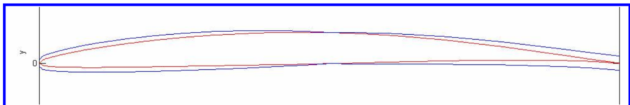
Fig.1 Changes in the thickness profile. The red line represents the original configuration, while the blue line represents the modified airfoil.
