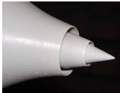
Fig. 3 Coordinates and picture of BPR10 nozzle
