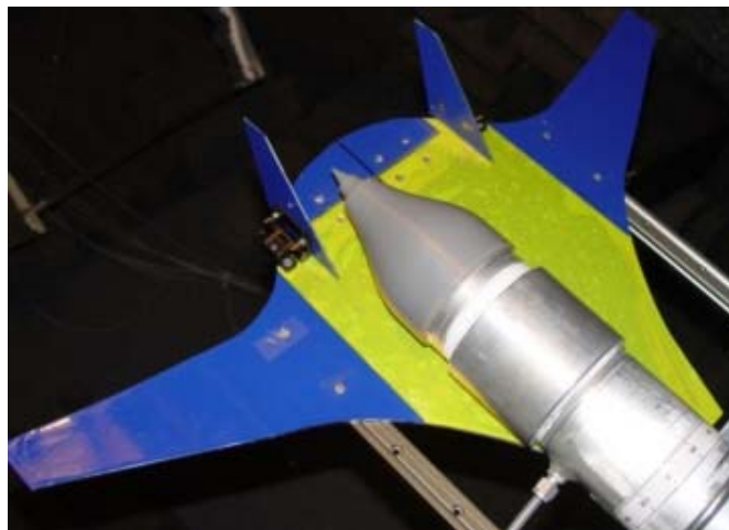
Fig. 2 Installation of nozzle and HWB shield.
