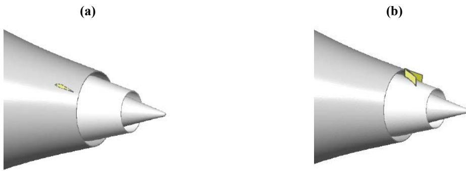
Fig. 4 Types of deflectors used: (a) internal vanes; (b) external wedge.
